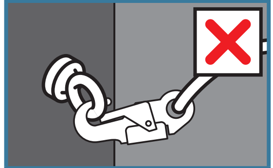
FIGURE 22 Roll-out on a small diameter eyebolt.
