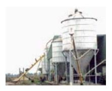
Silos with steep cones that ensure complete emptying and bottom inspection.
