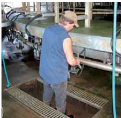
A rotary dairy pit, with removable grate, can reduce manual handling hazards by allowing for workers of various heights.
