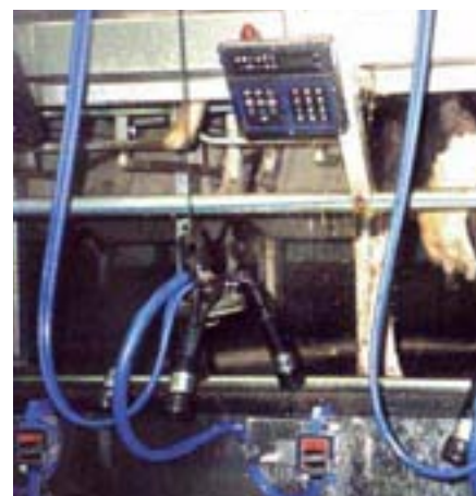
The cluster height on this ACR matches the needs of the operators.
